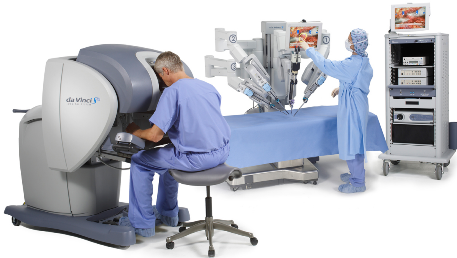
Figure 1.3: da Vinci Surgical System showing surgeons console, patient side cart and vision cart (©Intuitive Surgical, Inc.)
